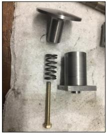
hard up against the top of the horn guides. I also understand from discussions at the track that a coil spring inside another coil spring should be wound in the opposite direction to stop coil locking. Eventually, I overcame this problem by carrying out a search on the internet and purchased longer springs which I am pleased to say have worked well once the loco was finished and put into service.
