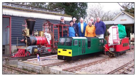
Our new ground level team member Dave is working on a new coupling design for the red ballast truck to replace the existing arrangement attached to the bogey which is often the cause of derailments when the wagon is empty. The new design will be fixed to the truck body and will solve this problem.
